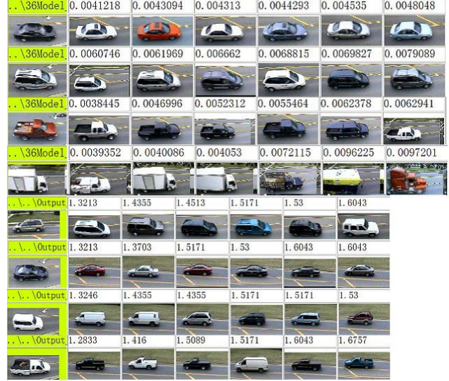
Figure12. Demonstration of object querying. The leftmost column shows the vehicle images used as queries. Each of the corresponding rows on the right show the vehicle objects returned as matches ordered from best to worst.
