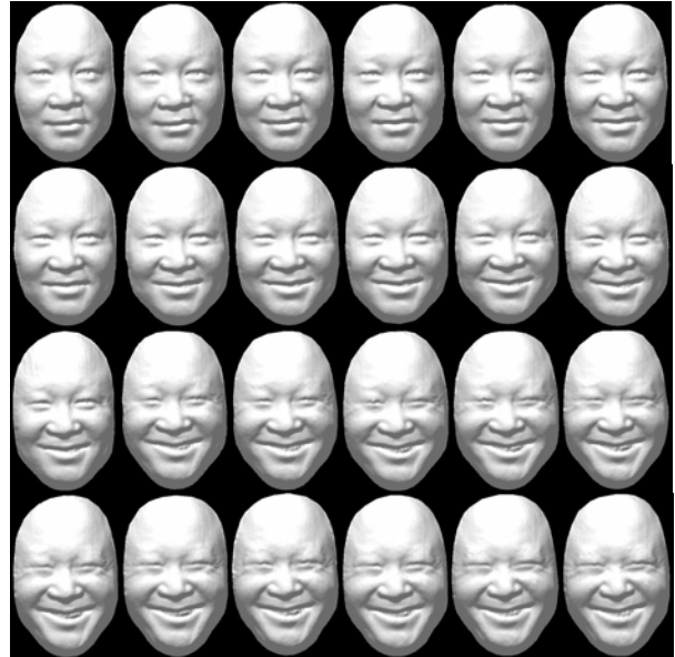
Figure 6. Sequence of measurement results of human facial expressions with the six-step triangular-pattern phase-shifting method.
