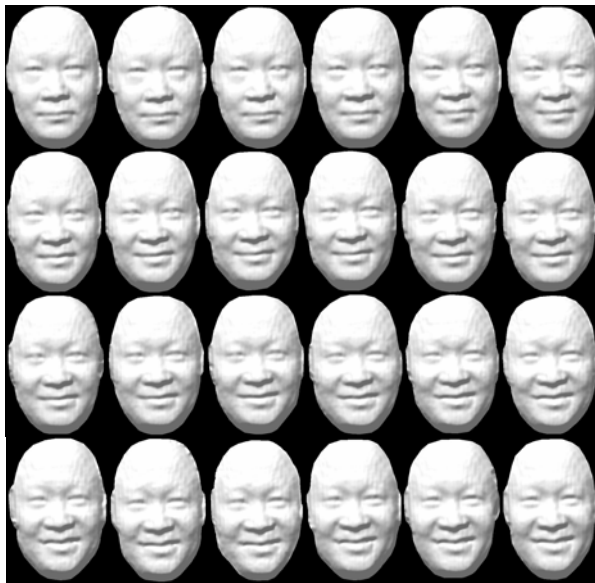
Figure 5. Sequence of measurement results of human facial expressions with the two-step triangular-pattern phase-shifting method.
