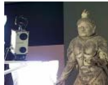
Figure 9. The scanning scene of the Koumoku-Ten clay figure using the VIVID 910
