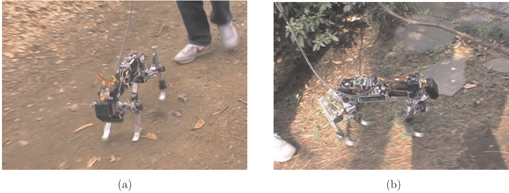
Fig. 1. Photos of Tekken2 walking on natural ground. The cable is just to prevent Tekken2 from damage in the case of an emergency, and is usually slack. The average walking speed was approx. 0.7 m/s.
