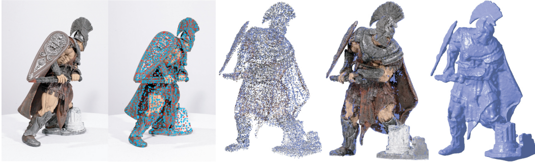
Fig. 1. Overall approach. From left to right: A sample input image; detected features; reconstructed patches after the initial matching; final patches after expansion and filtering; and the mesh model.
