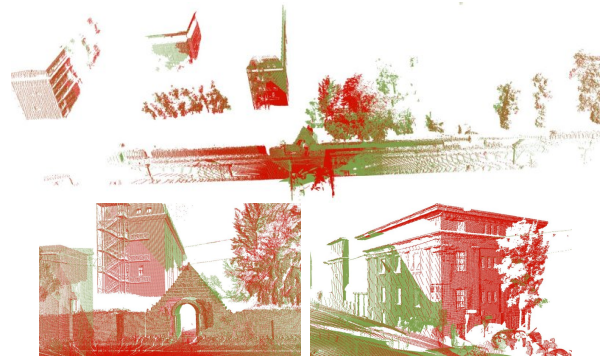
Fig. 10. Fine registration after SAC-IA, using a non-linear Levenberg-Marquardt optimization method. The two individual registered datasets are shown with red and green respectively.
