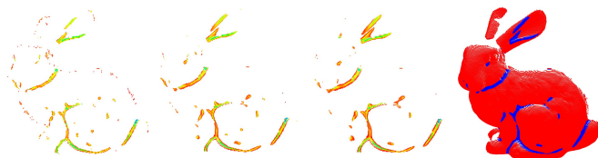
Fig. 2. From left to right: PFH persistence over multiple scales ( r_1 = 0.003 , r_2 = 0.004 , r_3 = 0.005 ) and the set of overall persistent points for the bunny00 dataset.
