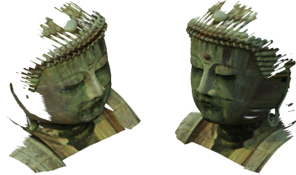
Figure 6: Aligned color texture on the 3D geometric model
