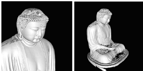
Figure 5: Merged result: The model contains 3 millions points and 5.5 millions triangles
