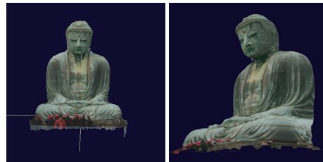
Figure 7: Aligned color texture on the whole body of the 3D geometric model
