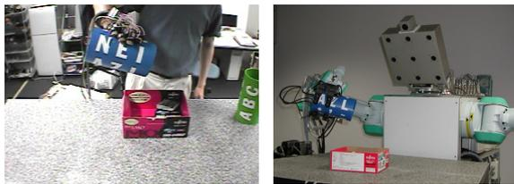
Figure 8: Human demonstration and robot performance. The pose of the robot arm in the right figure is calculated from the relative pose of the object in the left figure.
