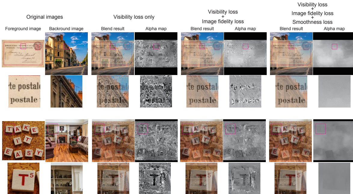
Fig. 15. Results of the ablation study of loss functions. The second and fourth rows show enlarged images of the areas enclosed by dashed lines in the first and third rows, respectively. (Second column) Results obtained using the visibility loss only. Without the image fidelity loss, patterns that do not exist in the original image are produced to achieve the target visibility. As a result, the visual quality of the generated images significantly degrades. (Third column) Results obtained using the visibility loss and image fidelity loss. The image fidelity loss ensures that the results retain the original image structure. However, in some cases, the gradient-based optimization can still be trapped in suboptimal local minima. (Fourth column) When the edge-preserving smoothness loss is combined, the aforementioned problems are resolved, and visually pleasing results are obtained. Input images are by 2211438 / Pixabay , Tama66 / Pixabay , Alexas_Fotos / Pixabay , and Mariamichelle / Pixabay
