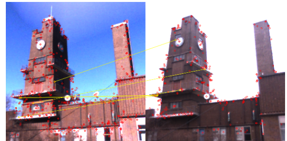
(a) SURF matching between input image and database image
