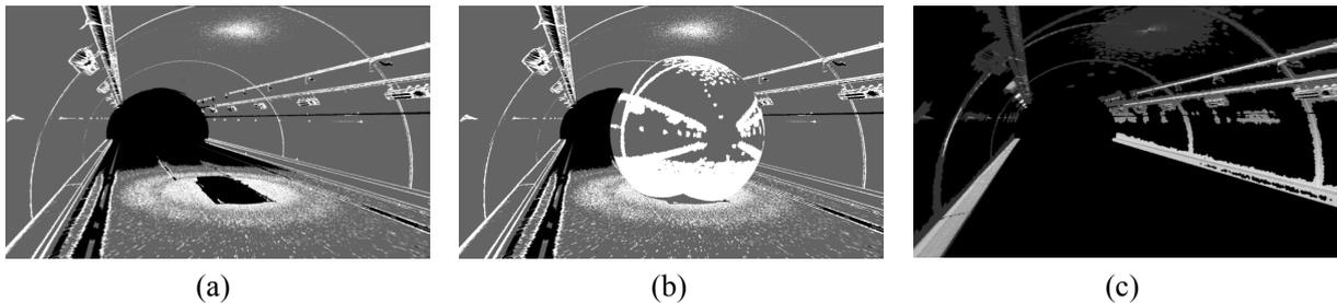
**Figure 3 – Edge extraction schema. (a) Highlighted edges. (b) Edges mapped onto a sphere and expanded. (c) Expanded edges displayed in the original position, with the road surface eliminated.**
