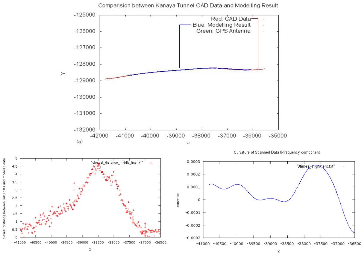
**Figure 10 – (a) Outer boundaries in CAD data and Inner walls in the 3D scanned model. (b) Difference between 3D model and 2D CAD data. (c) Curvature of the tunnel.**
