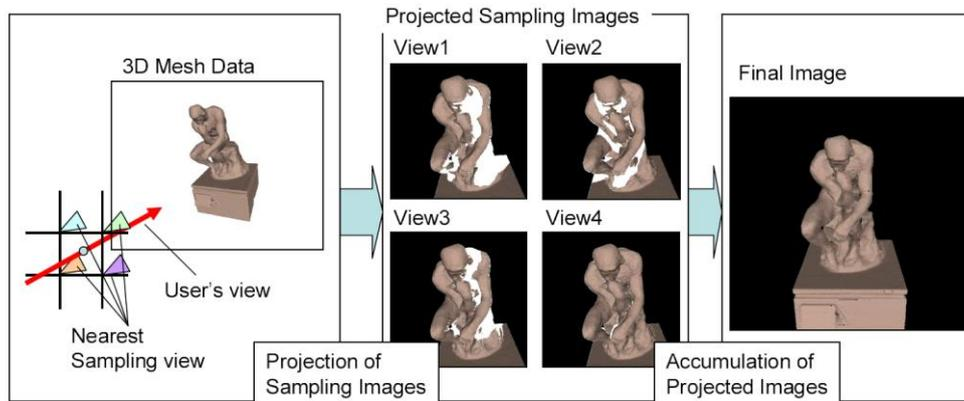
**Fig. 3** The reconstruction of images by projective texture mapping using GPU capability. We can efficiently extract each pixel's correct color from sampling images by texture projections. Each nearest sampling image is projected from the sampling point to the geometric data. By accumulating the results in the final buffer, we can obtain the reconstructed image
