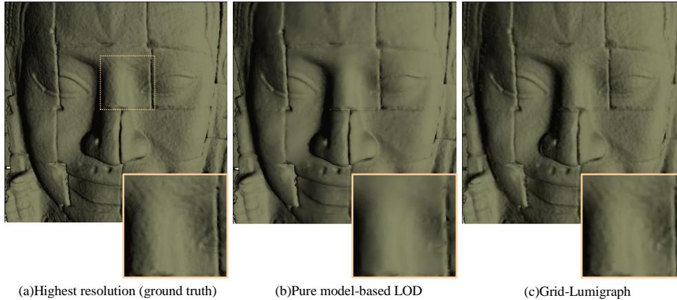
**Fig. 12** Comparison of the quality of images rendered by (a) highest resolution model, (b) pure Model-based LOD method, and (c) Grid-Lumigraph. Right bottom images are magnified views
