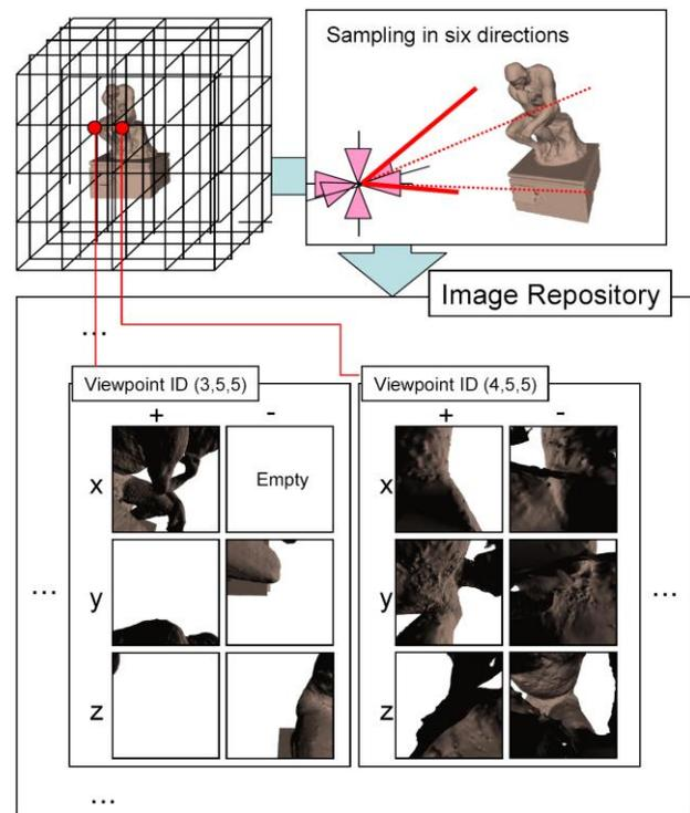
**Fig. 5** Sampling from each grid point. Viewpoints for sampling are located on each grid point of the voxel space surrounding the input 3D model. View directions are set along axes  $x$ ,  $y$ , and  $z$ . The image repository manages sampling images in a hash table.
