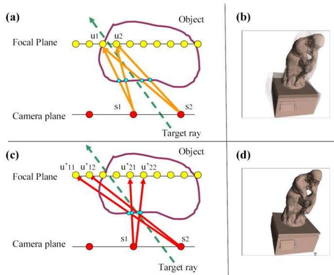
**Fig. 2** Correct sampling with geometric information. (a) Extraction colors from sampled colors without geometric information. (b) The result without correction. (c) Extraction with geometric information. (d) The result with correction using geometric information.
