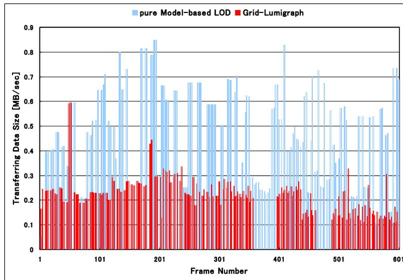
Fig. 11 Transferring data rate (megabytes per second) of pure model-based LOD method and Grid-Lumigraph
