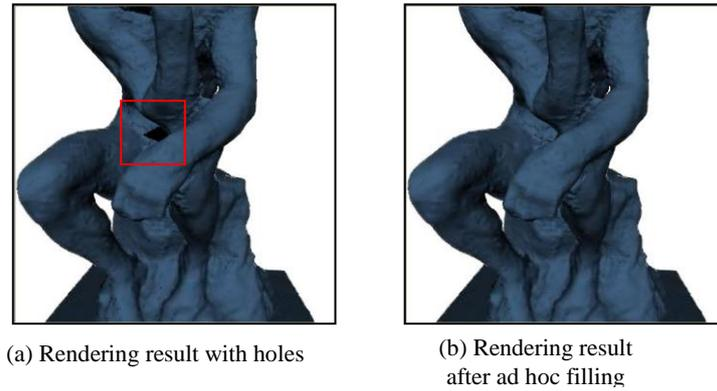
**Fig. 8** Filling holes. (a) is a rendering result with some holes because of the low sampling granularity. In the interactive time, the filling procedures are done ad hoc by using sparse model data located on the client as shown in (b).
