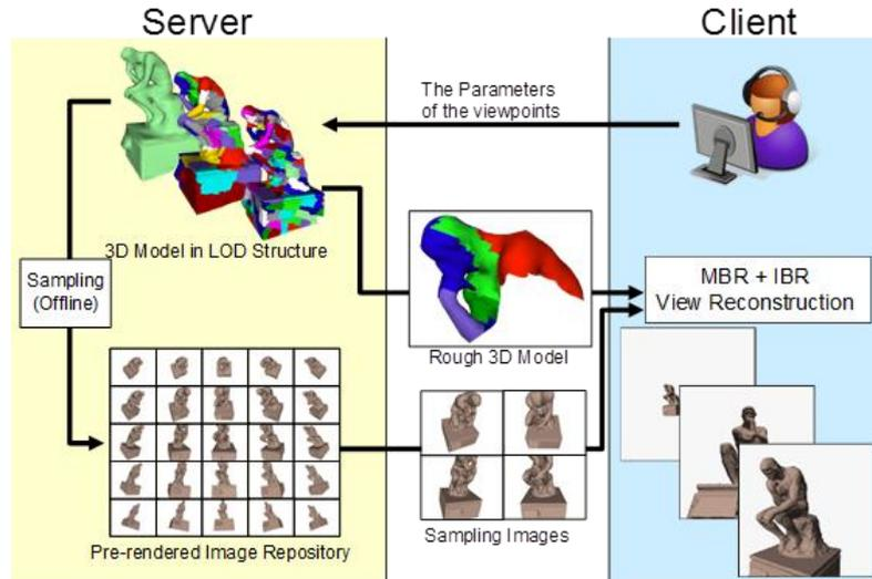
**Fig. 1** Overview of proposed rendering system. The server contains geometric data recorded in the format of an LOD hierarchy and the repository of sampling images of the input 3D model. The client system displays arbitrary views reconstructed by using received images and sparse 3D mesh patches.
