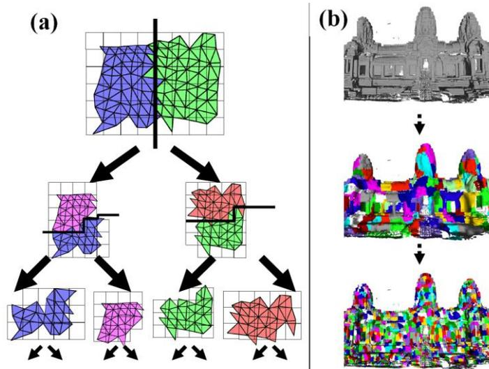
**Fig. 4** Construction of Level-of-Detail hierarchy.
