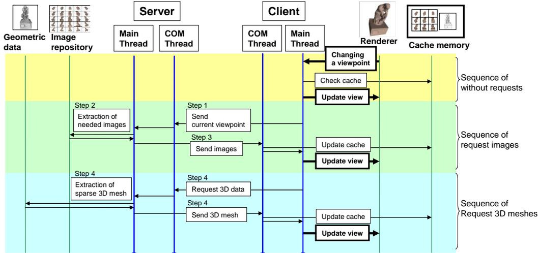
**Fig. 6** The sequence chart for the rendering pipeline on our system. If the client's cache has enough data to reconstruct the current view, the client's thread can display the view without requests to the server. Otherwise, the client makes requests for images and 3D meshes to the server. The data communication is managed by COM threads, and it is asynchronously done. The renderer updates the view whenever the data communication is finished.
