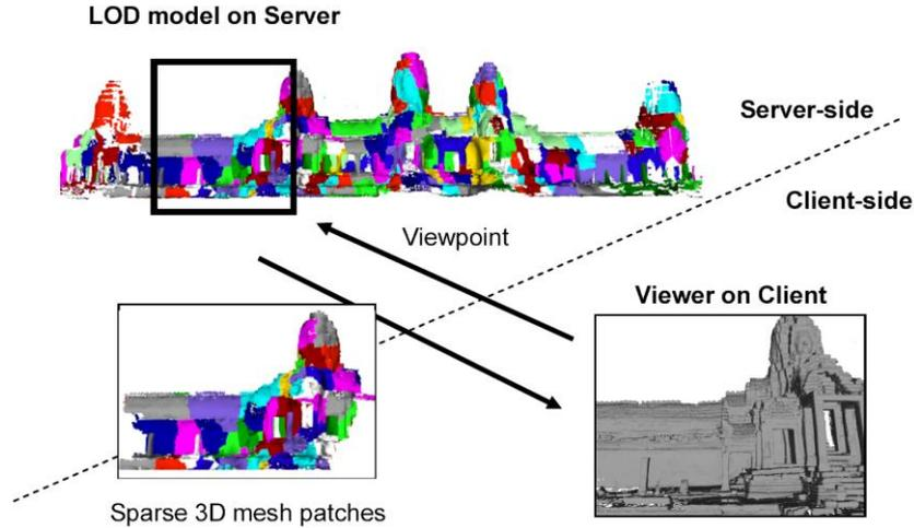
**Fig. 7** Communication of the geometric data. The server provides very sparse mesh patches depending on the client's viewpoint. The sparse mesh patches are chosen from the LOD hierarchy structure.
