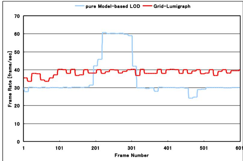
Fig. 10 Rendering speed (frames per second) of pure model-based LOD method and Grid-Lumigraph.
