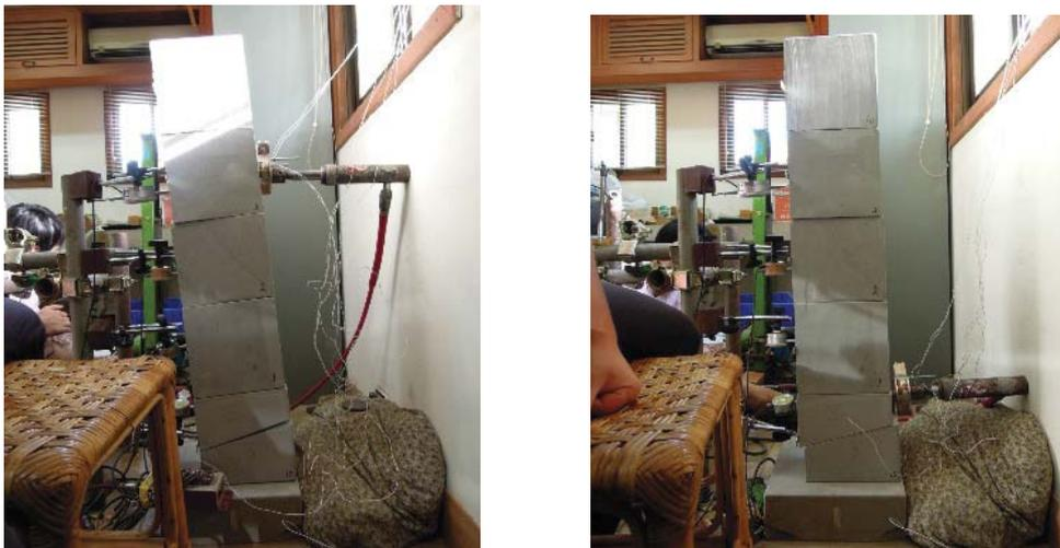
Figure 13: View of rotation mode and sliding mode.
