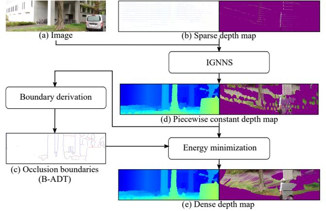
Fig. 2. Flow chart of our depth completion. (b), (d), (e) Left: depth maps, right: point clouds from a side viewpoint. (c) Colors indicates, white: not occlusion boundary, blue: vertical occlusion boundary, red: horizontal occlusion boundary, green: vertical and horizontal occlusion boundary. (d) In the piecewise constant depth map, all surfaces are parallel to the image plane. (e) Our energy minimization smooths depth within an object while preserving discontinuity at object boundaries.
