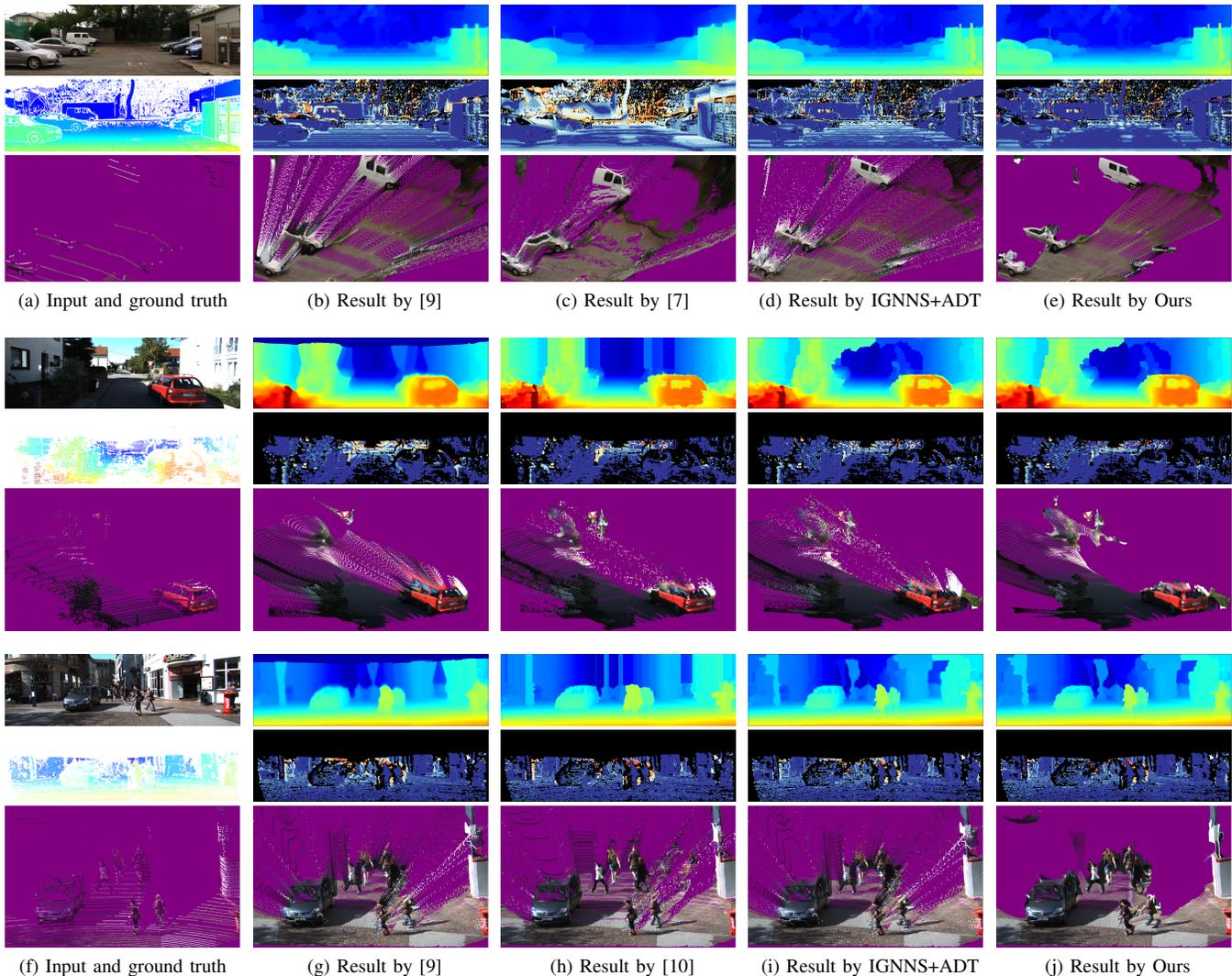
Fig. 6. (a) - (e) Results on a selected frame of Komaba. (f) - (j) Results on two selected frames of KITTI. (a), (f) From top to bottom: input image, ground truth depth map, and input LIDAR in point cloud. (b) - (e), (g) - (j) From top to bottom: depth completion result, error map, and depth completion result in point cloud. By comparing point clouds, we see only our method preserves the discontinuity at occlusion boundaries.
