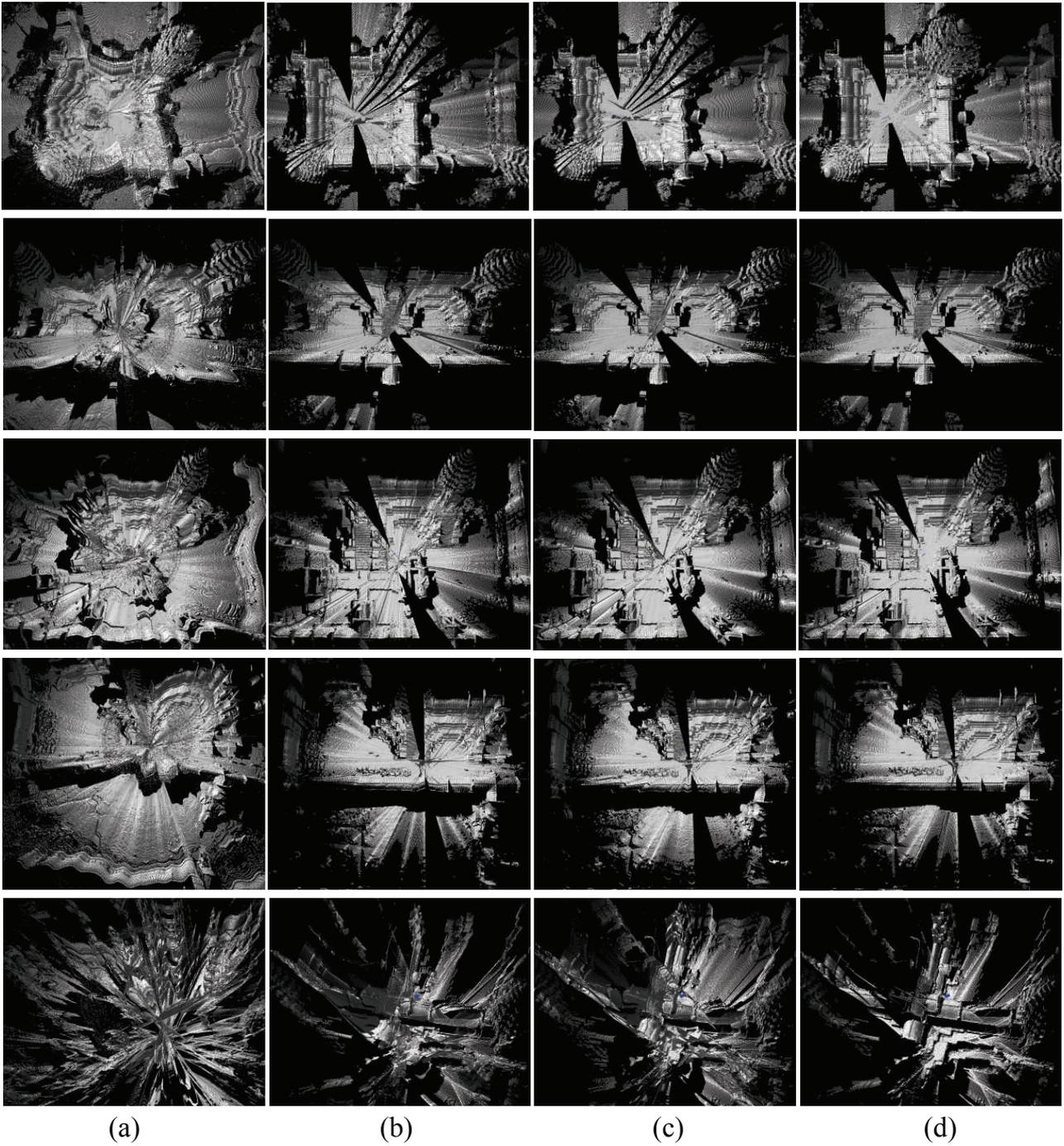
Figure 7. Comparison on data rectification: (a) raw data captured by laser scanner. (b) rectification using motion calculated by visual odometry [10]. (c) flying range sensor rectification [4] (d) our result.
