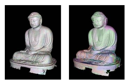
*Figure 3.* Synthesized range data. (a) Original whole mesh model of Kamakura Buddha, (b) Synthesized range data with initial perturbation and Gaussian noise to simulate alignment error and simulate sensor errors, respectively.
