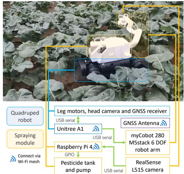
Figure 1. The quadruped robot scans for the worms on a raw broccoli field. The green arrows and the Wi-Fi mesh symbols denote the communication methods between different modules.
