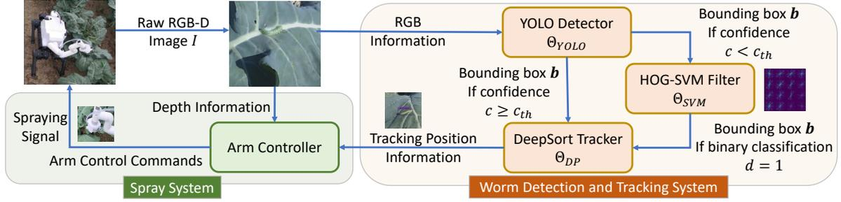
Figure 2. Worm tracking and pesticide spraying workflow overview
