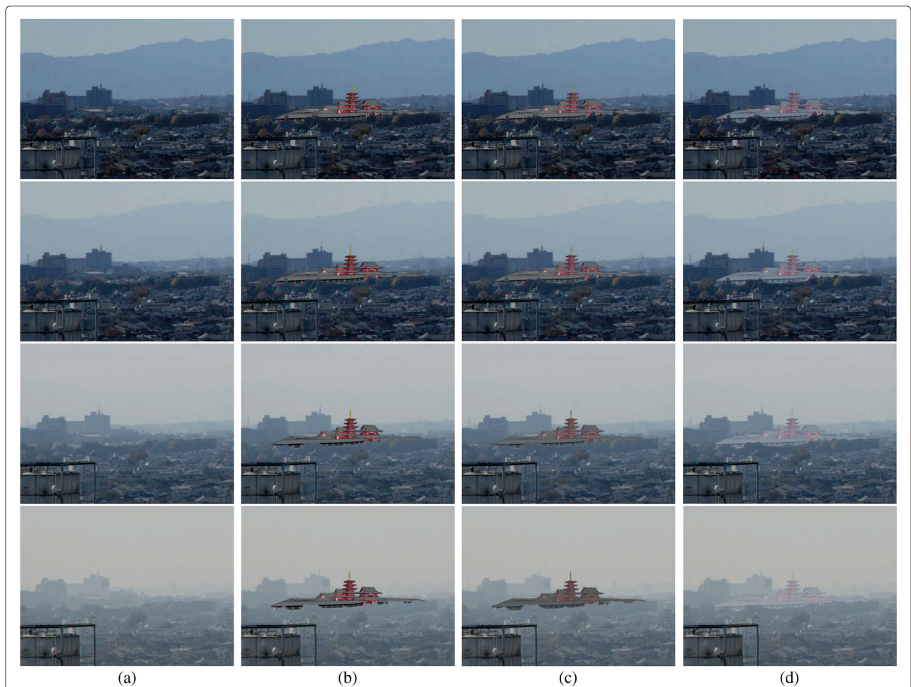
Fig. 14 MR application with aerial perspective effect. From top to bottom rows: scenes with turbidities T = 1.9, T = 2.11, T = 2.94, and T = 4.36 . a Input real scenes. b Virtual object without aerial perspective. c Results of [13]. d Our results
