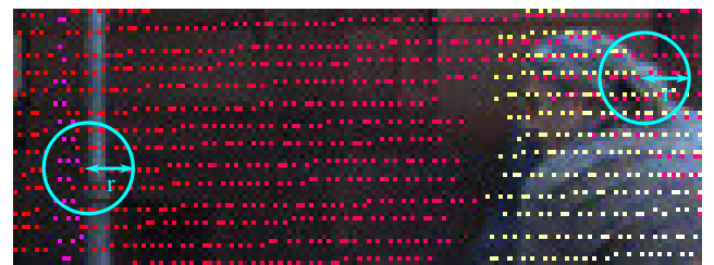
FIGURE 3. Candidate assignment of SSM. The circles indicate the areas to create the candidate sets for the centered pixels. Although there is mis-projection, the appropriate LiDAR values are located in the areas, e.g., purple for the pole at the left, and yellow for the person at the right.
