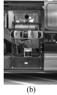
Fig. 7 The line scan camera and the laser range sensors mounted on our measurement vehicle. (a) the whole of the vehicle and (b) the line-scan camera and the scanning laser range finders.
