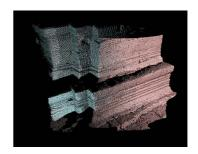
Fig. 8. The result of aligned range images: Red points represent the 3-D model obtained from a fixed sensor and light blue points represent the 3-D model obtained from the climbing sensor.
