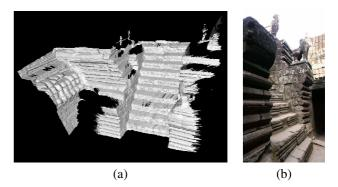
Fig. 7. (a) The result of the model obtained from the climbing sensor by placing the horizontal scan in an interval calculated from the vertical scan. (b) Actual scene of the target.
