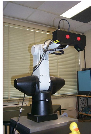
Figure 8: Robot Mounted Scanner
