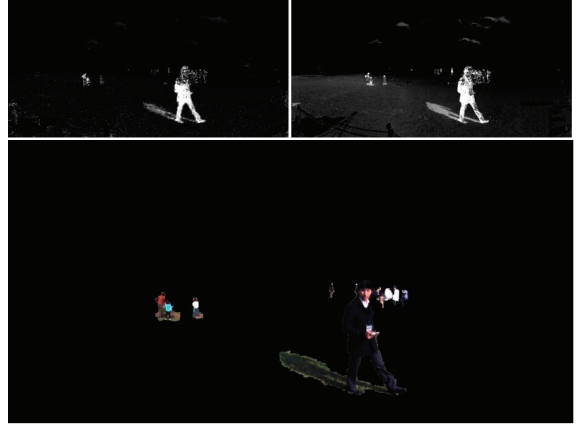
Figure 6: Result of illumination constraints. The upper left image shows the illumination invariant distance while the one on the upper right shows the illumination ratio distance. The whiter the pixel is, the larger the distance is. The lower image indicates the final segmentation result.
