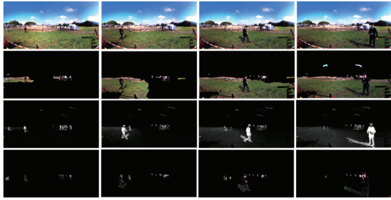
Figure 11: Asuka sequence. The images in the first row are original ones. The second row shows how the previous approach fails. The third row indicates probability of foreground from illumination constraints. The bottom row shows the results by our approach.
