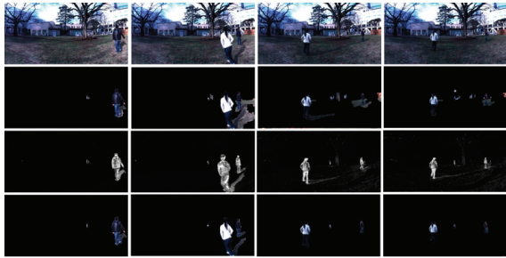
Figure 12: Campus sequence. The images in the first row are original ones. The second row shows how the previous approach fails. The third row indicates probability of foreground from illumination constraints. The bottom row shows the results by our approach.
