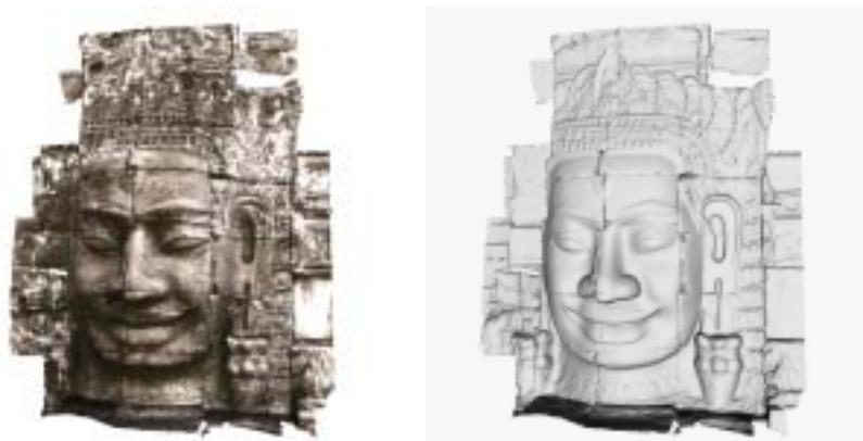
Fig.4 left: picture of face, right: measurement result of 3D face model
